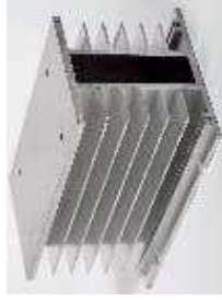
Model: MW-H-150 Size: 150mm*80mm*80mm For 60 amps SSR Mounting method: Panel mount and din rail mount Compatible with 8cm*8cm fans
