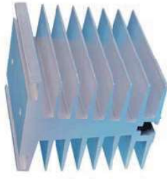
Model: MW-T-80 Size: 80mm*80mm*70mm For 80amps, 100amps, 120amps Mounting method: Panel mount or din rail mount with din rail adaptor
